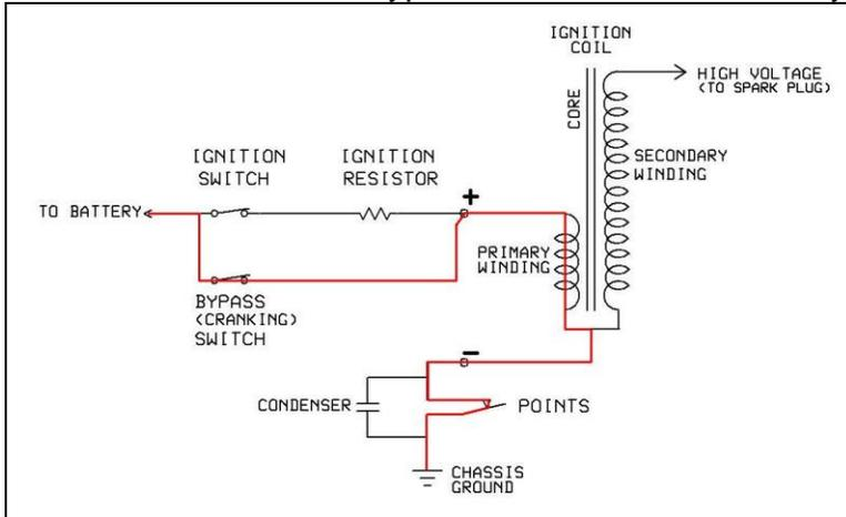
Current flow while running – Bypass switch off, current flows through the resistor reducing the voltage (typically 6 – 9 volts) to the coil when the points are closed
