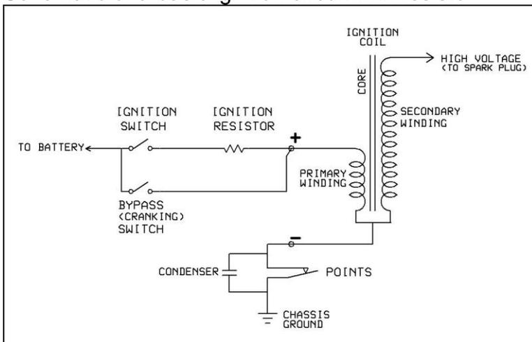
Current flow while cranking – Both switches closed (ignition and bypass) current takes the path of least resistance and bypasses resistor. Full battery voltage to coil
