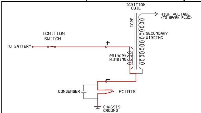
Current flow when the points open – Magnetic field collapses creating high voltage in secondary coil. Current flow is momentary - only for the duration of the spark.
