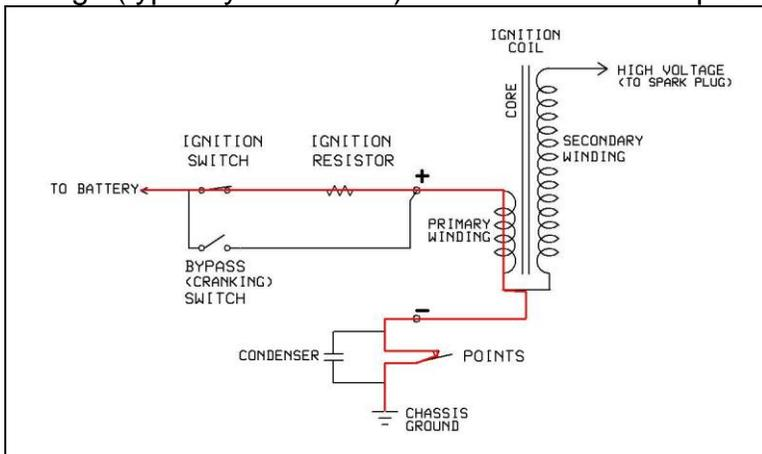
**Note:** When the points are open, no current is flowing through the resistor so there is no voltage drop. Consequently full battery voltage (12 volts) will appear at the “+” terminal of the coil when the points are open.
