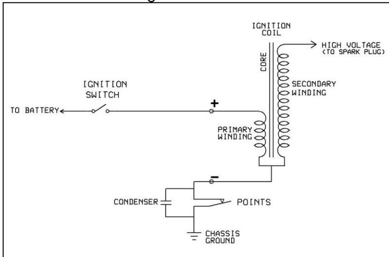
Current flow when the points are closed – Primary coil creating magnetic field
